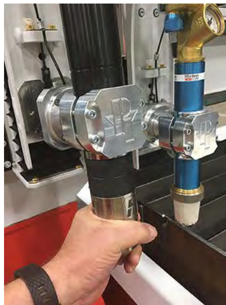
Magnetic collision mount disconnected from receiving plate
