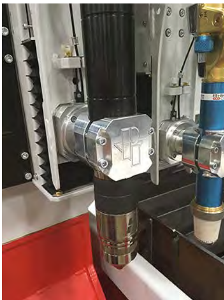
Magnetic collision mount attached to receiving plate
