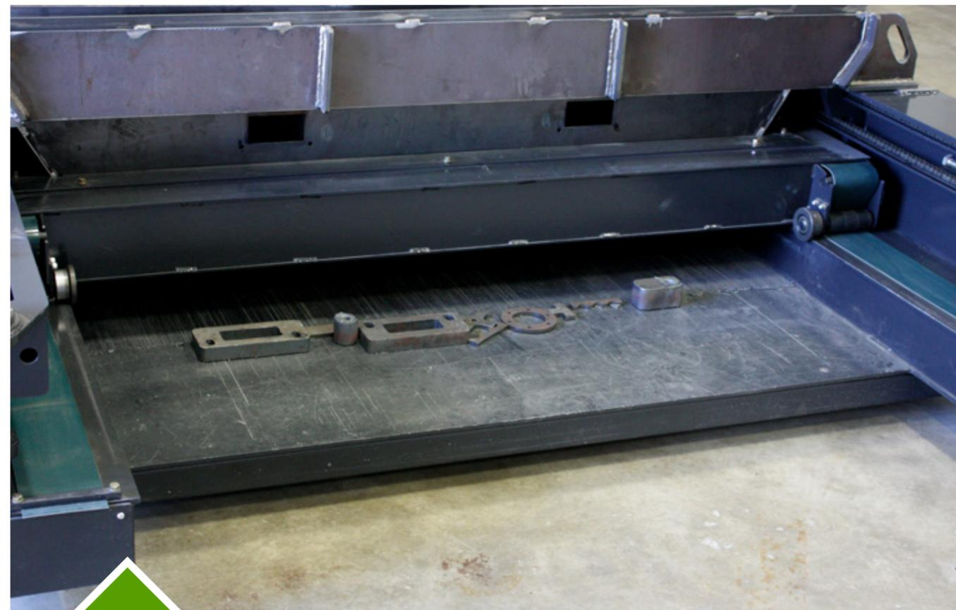
Unlike a conventional plasma cutting table with caked-on slats, like the one shown on the previous page, a TracKlean table with cleaning plow pushes slag and fallen parts to the front of the table.
