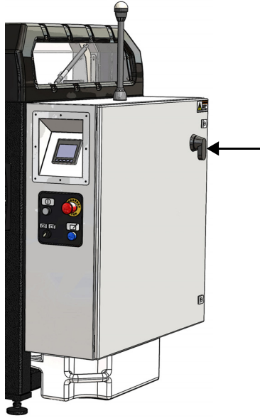
Primary breaker disconnect lever
