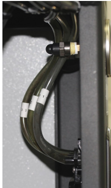
Good tube routing
