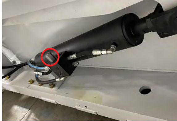
Relief valve located on top (or bottom) of cylinder manifold
