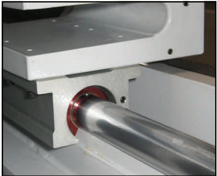
Close Up View of a Upper Bearing and Rail
