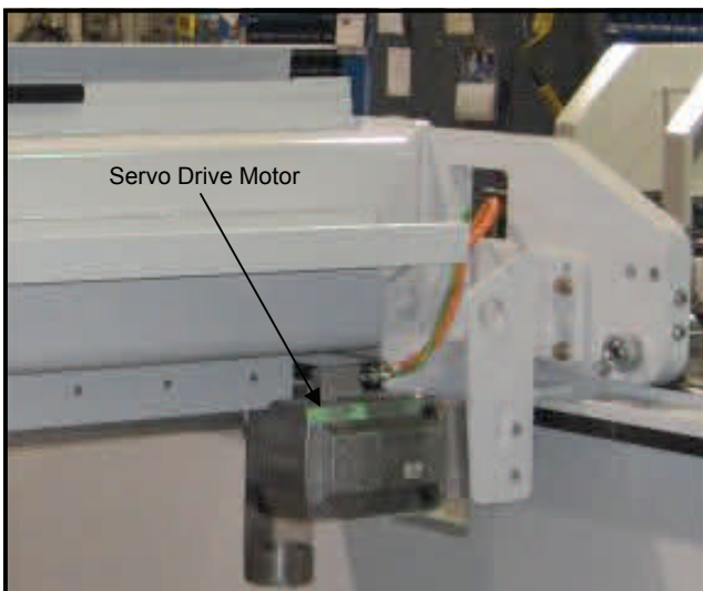
Away Side Gantry Drive Area
